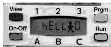
Figure 2: LCD, four buttons, and port labels.
