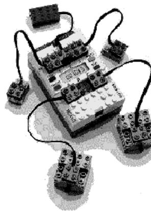
Figure 1: RCX attached with two motors (ports A and C), two touch sensors (ports 1 and 3), and a light sensor (port 2).
