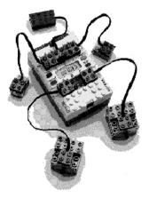
Figure 1: RCX attached with two motors (ports A and C), two touch sensors (ports 1 and 3), and a light sensor (port 2).
